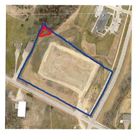
Red area above is a portion of Loess Hill slope. This area is not proposed for grading.
